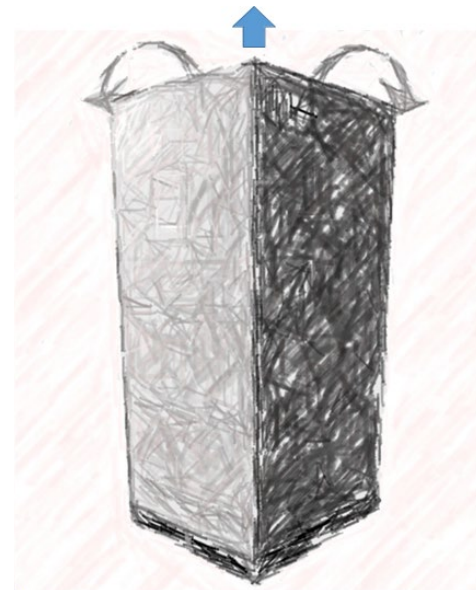
Image: Remove the covers. Start with the top and then remove the covers on the sides.
