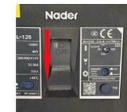
3. Lift the switch to switch on the station
