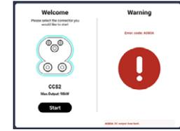
4 If an error causes the preparation to fail, an error message is displayed on the preparation page and only for the connector to be prepared.
